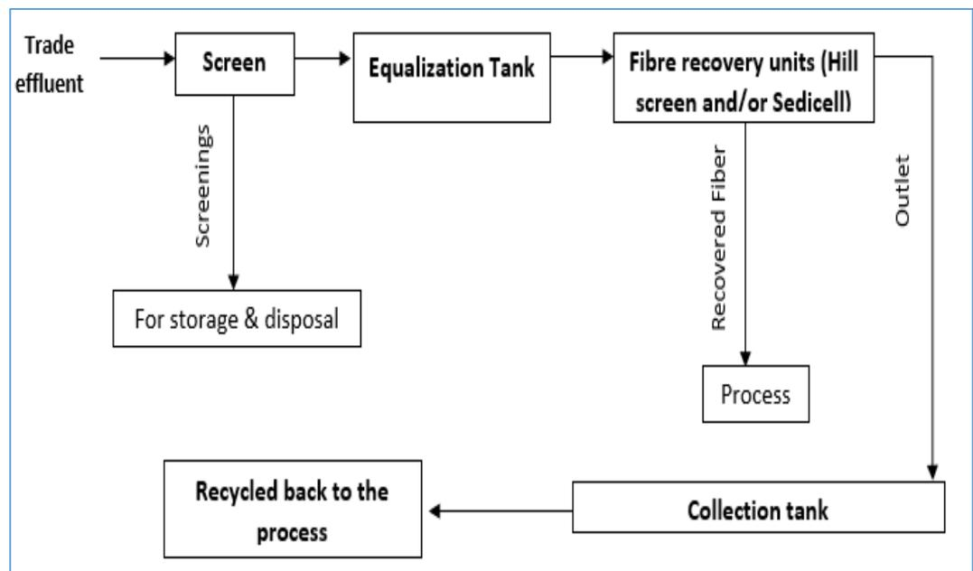
**Figure 1: Effluent management scheme in wastepaper based industries operating on ZLD (recycling effluent after Fibre recovery system)**
